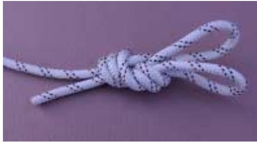
Figure 6 Double figure-of-eight on a bight
